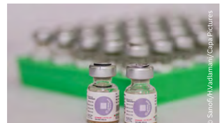
The purple symbol on this cholera vaccine vial from Sanofi changes colour through exposure to heat, to indicate whether the vaccine is safe for use.
